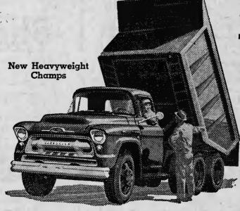
High-powered V8's-standard in heavy-duty jobs! You get the big new 322-cu.-in. Loadmaster V8 in 9000 and 10000 series trucks. The Taskmaster V8 is standard in other L.C.F. and heavy-duty models.
