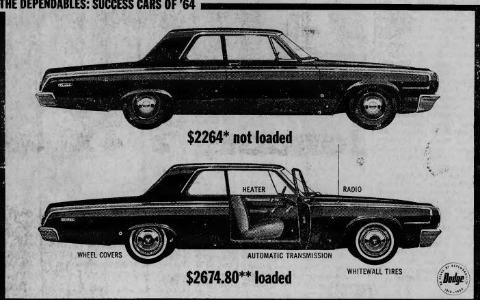
sedan. It has a unitized, rust-protected body, front seat belts, an alternator electrical system, self-adjusting brakes and a 225 cubic inch, six-cylinder engine. It will go 32,000 miles between major grease jobs, 4,000 miles
