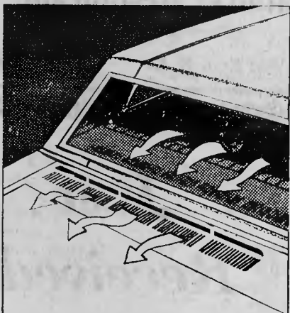
Silent-Flo Ventilation (on 4-door hardtops). Fresh air is drawn in, stale air removed even with all windows closed.
