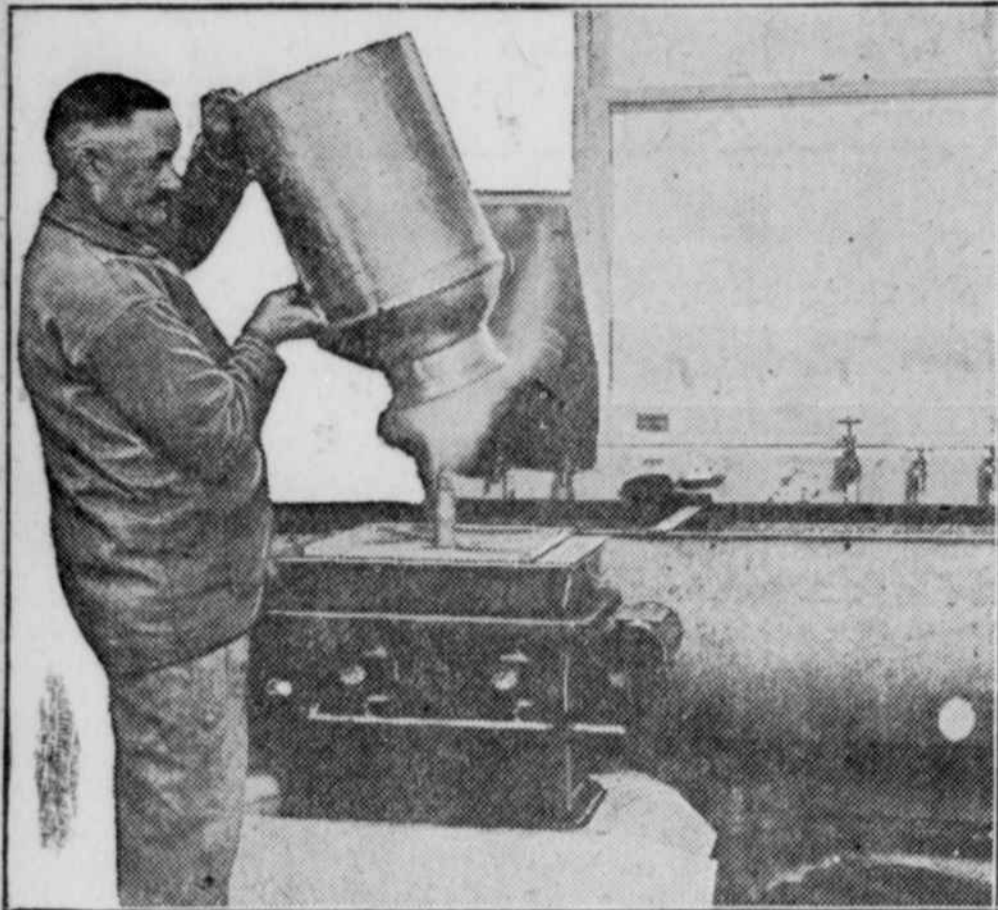
Placing a Milk Can Over the Home-Made Sterilizer—It Can Be Used on the Kitchen Stove.
