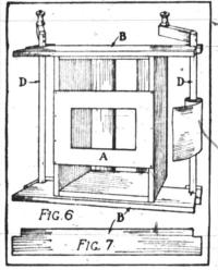
are driven into the roller, after the roller ends have been slipped into their pockets. Their purpose is to keep the rollers from slipping up or down (Fig. 6).
