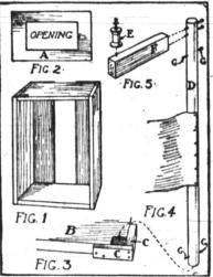
hold the rollers in the notches. Nail boards B to the two ends of the box an inch beyond the front edges of the box, and with the pair of roller pockets in the upper board directly over the pair in the lower board.
