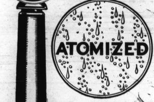
atomized mixture of gasoline vapor with liquid drops of raw gasoline. These rops, resisting the action of the spark, make starting difficult and cause uneven, sluggish power.
