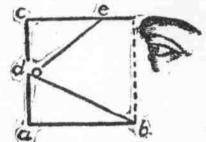
shows. Line A-B represents the bottom, A-C the rear wall of the box, D-L the slanting piece of pasteboard and D-E the slanting piece of looking glass. In the centres of the front and back sides of the box round openings are made; one for the eye, the other one to admit a marble, which is to roll down the slanting marble roll down and look into the box at the same time you will see the marble roll upward!
