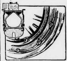
Combination of Steel Bands and a Rubber Cushion, Protecting a Pneumatic Tube, Constitute the Chief Features of This Puncture-Proof Tire and Resilient Wheel.
