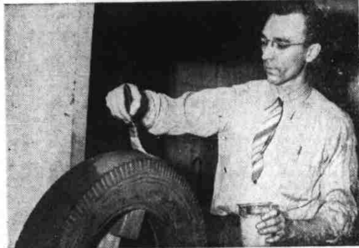
John Lange, is shown painting synthetic rubber liquid on an old tire at Trenton, N. J. Any number of coats of this new liquid may be applied to a smooth surface tire, each coat to be put on after the previous covering has dried. After it has dried, it is claimed that it will stand up well and give satisfactory additional mileage. (Central Press)
