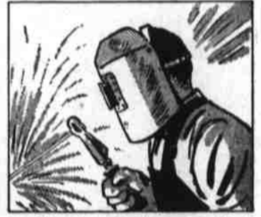
4. The helmet he wears is to protect him from light! The rays from a welder's arc could cause blindness if he did not wear this strange headgear.
