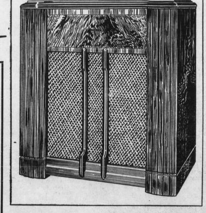
MODEL 30 BC - A 7-tube, including rectifier, radio-phonograph combination with automatic record-changer. Plays 14 ten-inch or 10 twelve-inch records. Chassis features include: 3 bands, 3-gang condenser, "push-pull" audio, 10-inch speaker, full range tone control, rotating Heliscope loop aerial, bass compensation.
