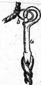
contrivance is quickly fastened or unfastened, and when not in use can be hooked into the staple with which the rope is attached to the hitching post. Nothing is more serviceable or economical for a temporary fastening where the farmer has no stanchion.—Harry Knowles.
