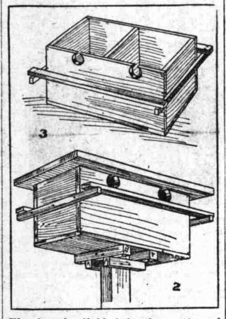
The box is divided in the center of its length by a partition, and a doorway is cut through one side of the box into each of the two compartments thus formed (Fig. 3).
