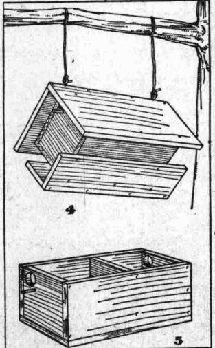
Nail a pair of cross pieces to the bottom of the box at a distance apart equal to the width of the post, and drive nails through the sides of the cross pieces into the post. There as a brace to these cross pieces nail another pair of cross pieces to the opposite sides of the post so their ends will come directly under the ends of
