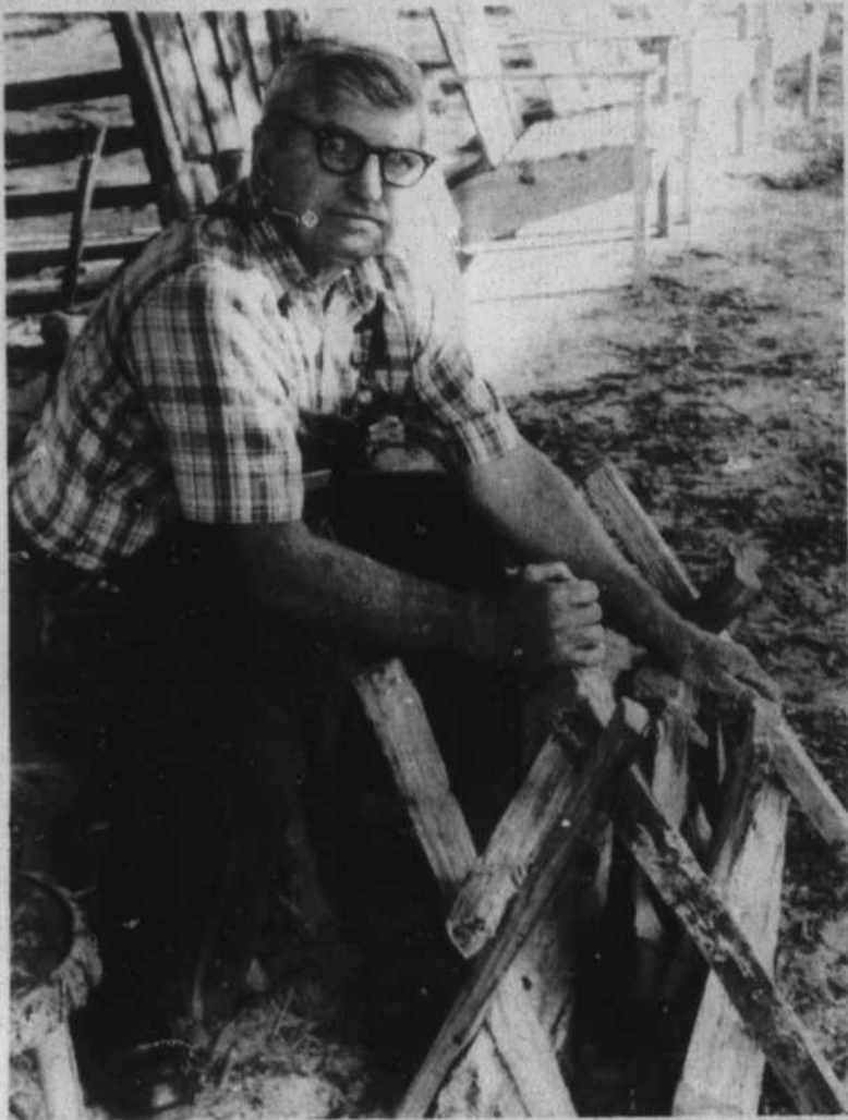
SPLITTING WOOD FOR MAKING SHINGLES
