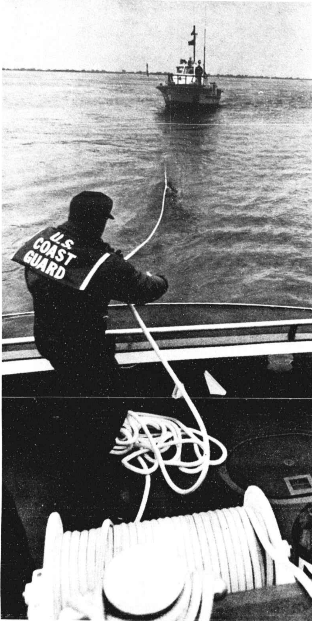
KEEPING IT TIGHT , a Coast Guardsman takes in slack on the tow line connecting his 41-foot patrol boat and the 44-foot motor lifeboat.
