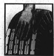
Rub your hand over this amazing Brake-Action Tread. Feel the extra safety in the sharp, biting edges of those 2500 "grippers" set at the angle of greatest resistance to forward and side skids!
