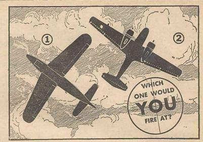
NOT AT NO. 1! It's one of Britain's best naval planes, the Fairey "Fulmar," a two-place, low-wing fighter. The leading edges of the wings of this plane are swept back sharply. The trailing edges are swept back also, but at a smaller angle. The long nose and fuselage are tapered to a point. The tapered tailplane has rounded tips.
