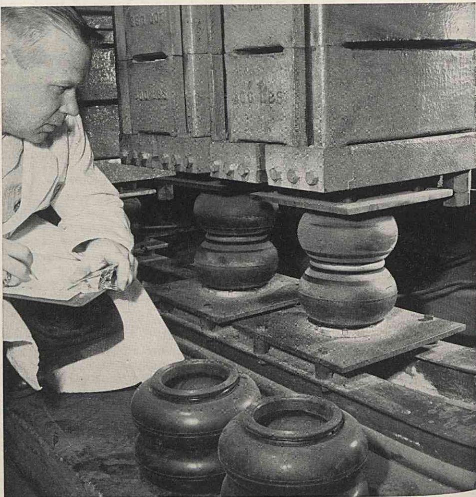
PRODUCTION OF AIR SPRINGS FOR BUSES WAS STARTED DURING THE YEAR. IT APPEARS THAT THIS NEW METHOD OF SUSPENSION FOR MOTOR VEHICLES WILL GAIN WIDE ACCEPTANCE IN THE AUTOMOTIVE INDUSTRY.
