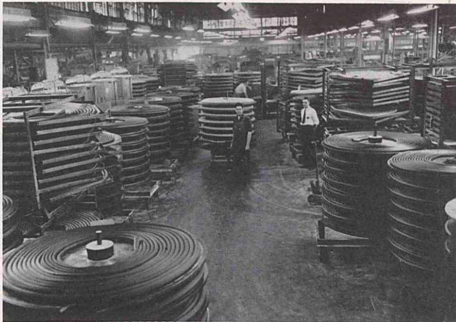
**ROLLS AND ROLLS OF HOSE**—The Noblesville plant manufactures a substantial percentage of radiator hose used by the automobile industry. The picture above shows hundreds of coils of extruded radiator hose tubing.
