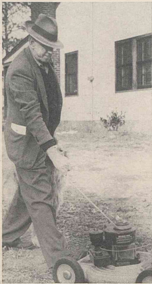
A ROTARY LAWN MOWER last summer jumped at Jeff Galloway, Carding, but the blade didn't cut through the steel plate in his safety shoe. Here demonstrated is the unsafe practice leading to the accident which could have been serious.
