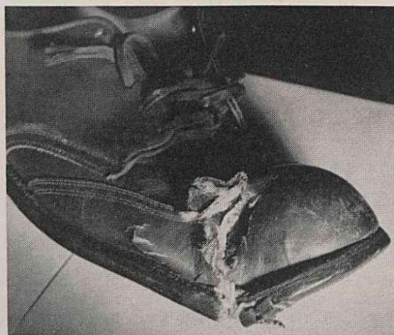
**A CLOSEUP** of the damaged shoe. The mower blade was stopped by the steel toe plate.
