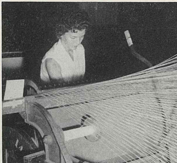
YARN must be transferred from packages to large beams, to go to looms for weaving into fabric. Cloe McDaniel, third shift for five years, operates warper.
