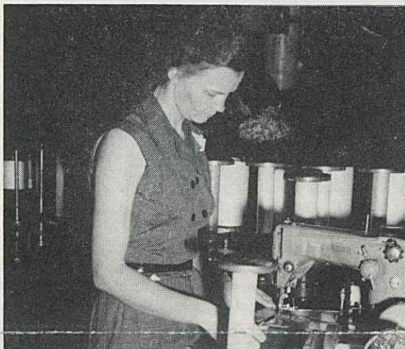
SPLICING synthetic cord with automatic sewing machine: Marjorie Anderson, on third shift for ten years.
