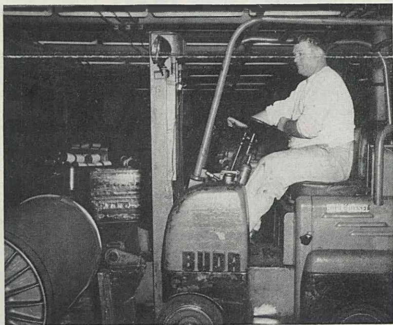
INCOMING synthetic filament, bought from suppliers, begins long journey through twisting, winding, spooling and weaving processes. It will emerge as fabric that helps give Firestone tires their long-wearing, safety features. Here, William Holton, fork truck operator, transports beams from warehouse to plant.
