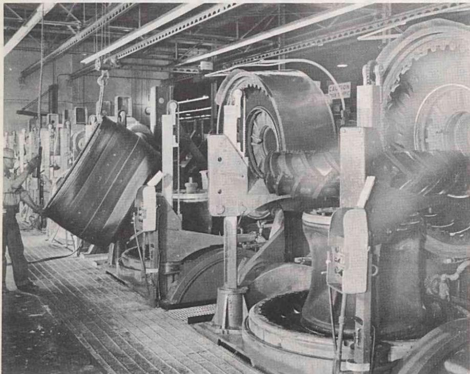
**ADDITIONS AND IMPROVEMENTS** to plants and equipment amounted to \$48,476,032 during the year. At the Des Moines plant, for example, this new line of 75-inch automatic bladder-type presses was installed for the curing of agricultural tires.
