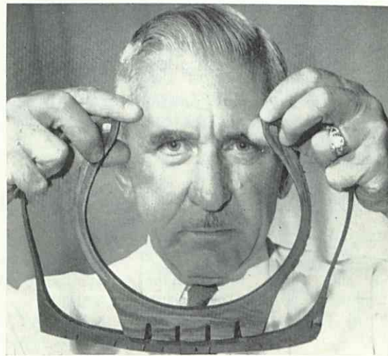
• Engineer Cory shows thin sidewall section was cut from a Firestone Indianapolis tire, while section with thick sidewalls was from a special tire for taxis doing low-speed city driving. At turn-pike speeds, a tire as bulky as the heavier one would fail because of excessive heat it would create.
