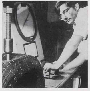
16,000 **POUNDS** • This steel plunger is one of many instruments TORTURE used in testing modern passenger tires. The plungger here is capable of up to 16,000 pounds pressure. Device is forced into tread of a Firestone Radial V-1 steel-belted tire to measure strength of tire's cords as well as its overall construction.
