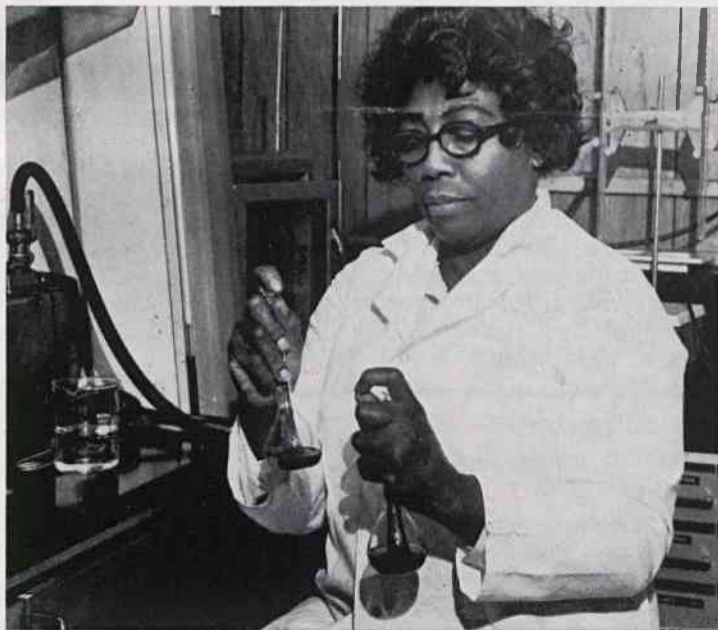
• Ida Byers making a chemical analysis to determine the zinc-copper balance of brass coating on steel tire cord.
