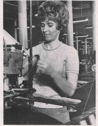
· In splicing reclaiming, short "mill-end" lengths of plied tire cord are transferred from small or scant spools to full spools suitable for creeling and weaving into fabric.
