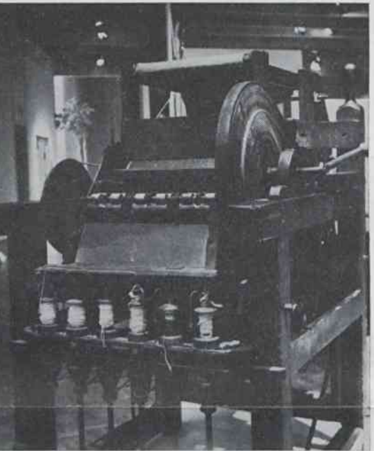
1764, the Arkwright frame was one of the first machines that enabled production of more than one thread at a time. Original Hargreaves' Jenny was hand-powered.
