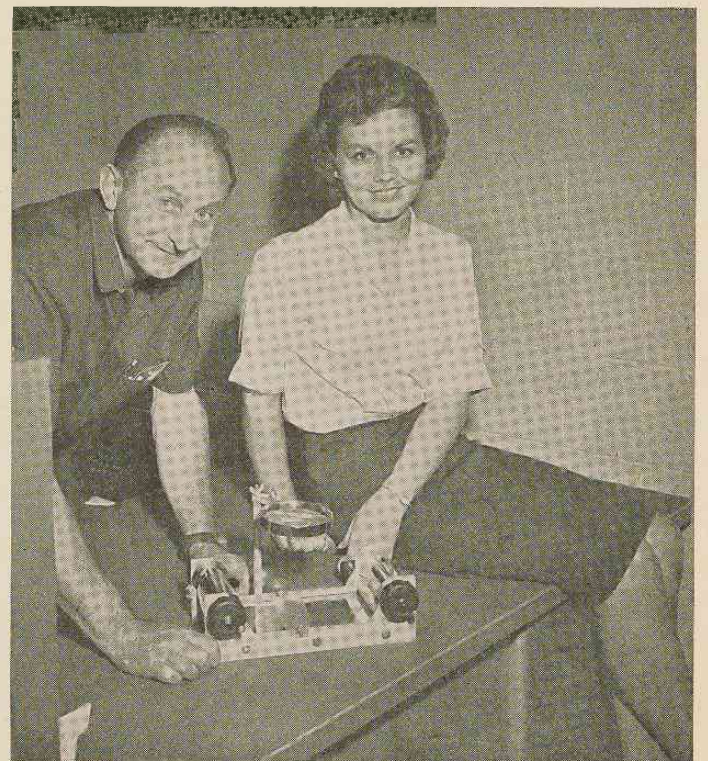
That Rube Goldberg-looking device that Engineering Liaison F. L. Sfreddo is demonstrating to secretary Barbara Trivette serves a very serious purpose. It's name is a Data Redoubt Unit, and its function is to aid in the reading of tapes from in-flight recorders now installed on all F-27's. The tape, made from fire resistant stainless steel, shows altitude, air speed, compass heading, and vertical acceleration. The information is kept for 60 days. If there is an accident within that period the FAA uses the tapes to help determine the probable cause.
