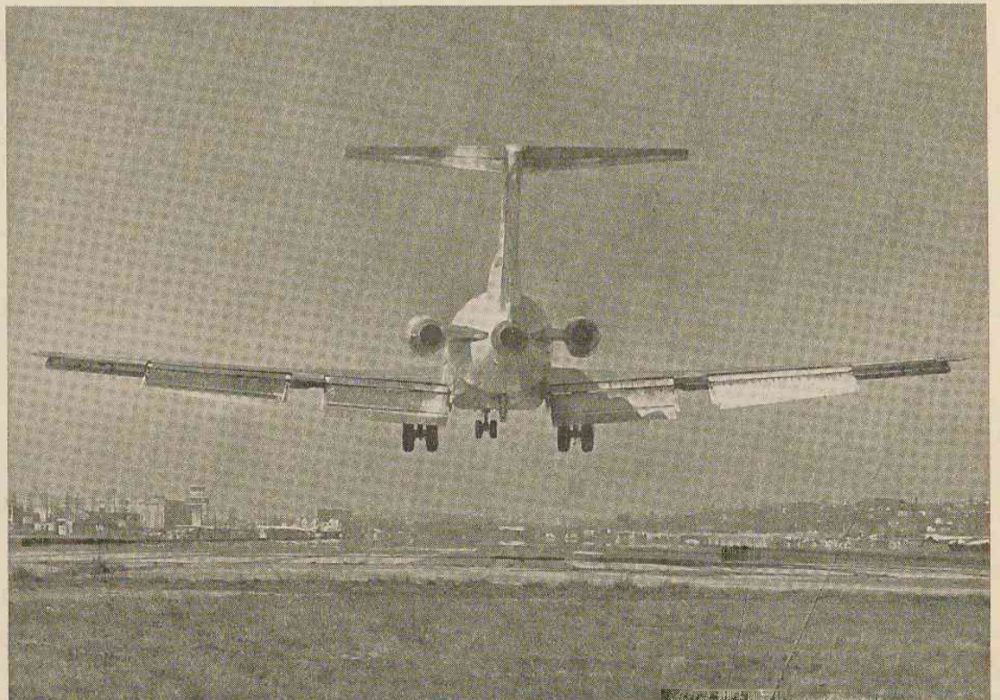
The Shape of Things to Come — This Boeing 727 is shown on its first flight test during which it was aloft two hours, three minutes. The aircraft, with three rear-mounted jet engines, will have one of the most extensive test programs ever given a commercial airliner. Total orders for the 727 now stand at 131 airplanes for seven airlines, with deliveries to begin later this year.
