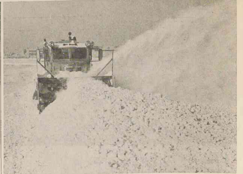
The CMH "Sno-Go" sends snow flying up to 30 feet in the air. Winter equipment can have Port Columbus ready for business in 30 minutes.
