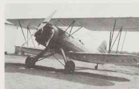
The Waco UP F-7 was used in the CPT program and for acrobatic instruction. The biplane accommodated only the pilot and his student.
