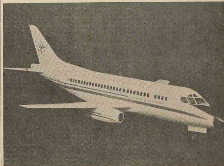
NORTH AMERICAN AVIATION'S CENTURYLINER is easily adaptable to varying passenger-cargo configurations. A moveable bulkhead makes possible almost any combination.
