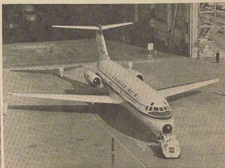
THE DOUGLAS DC-9 is designed to operate over segments of 100 to 1500 miles at the same speed and comfort as the larger jets. This aircraft, like the 111, has been tested and could be delivered in 1966.
