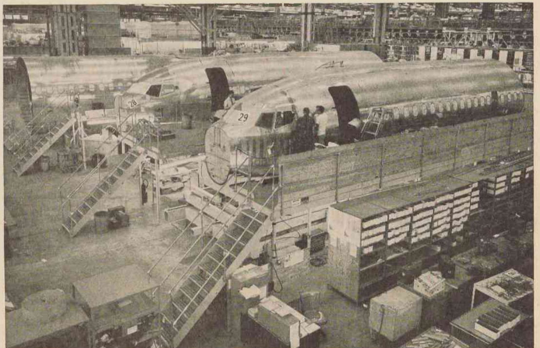
PIEDMONT'S FIRST Boeing 737 forward fuselage is shown here taking shape at Boeing's Wichita division. Since this picture was taken both this section and the rear fuselage half have been shipped to the
