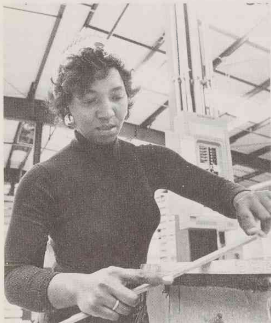
Filing, to Vera Taylor, has nothing to do with putting papers in a folder. She files to a smooth finish the furniture's formica edges.
