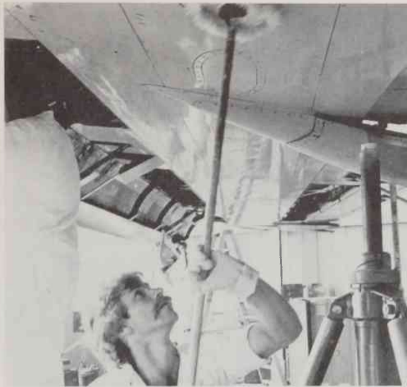
Don Newsome uses a plain but proven mop and special soap to wash the bottom of a 727 wing. Exterior washing is the first step in the aircraft cleaning procedure.
