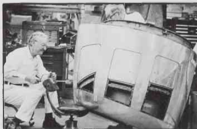
Repairing of the engine nose cowl is done by Harold Wooten (left) and Dewey Meadows, Sheet Metal mechanics.
