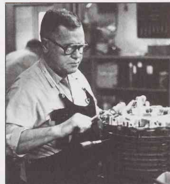
Mechanic Norman Shelton, one of 60 employees at the IND hangar, bleeds a DC-9 brake at the brake and tire shop.
