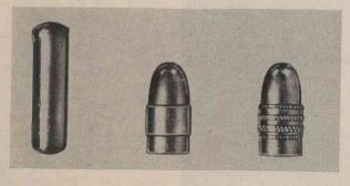
Extruded led slug Finish swage slug Knurled bullet
