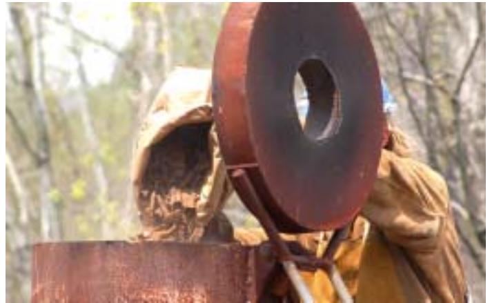
Josh Carter empties a 40 lb charge of broken iron into the furnace.
