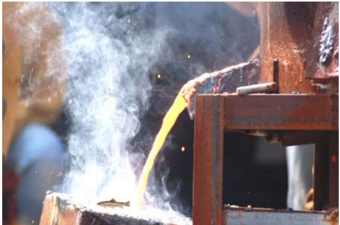
Orange-colored iron flows from the copula into the ladle at a temperature around 2750°F.
