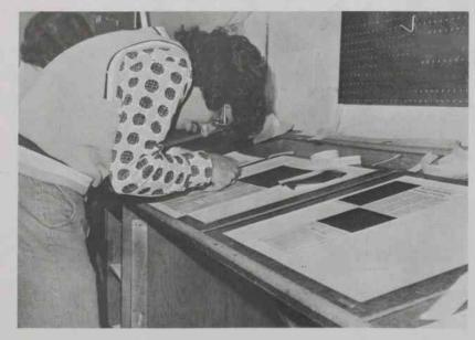
While the phototypesetter was at work a layout man has made up a "dummy", or a rough draft of what each page will have. He now assembles the articles on a sheet of paper, exactly as it will appear in the paper.
