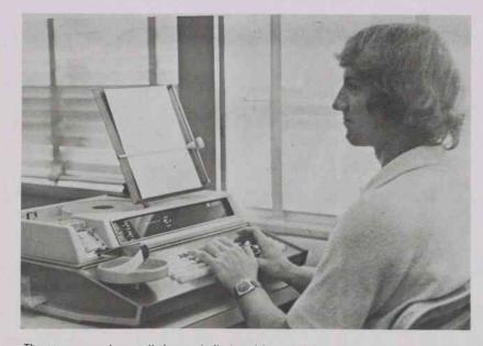
The newspaper story, called copy, is first sent to a phototypesetter. Using a machine similar to a typewriter, the phototypesetter punches the article on paper tape, using a code of punched holes. Each letter and command has a specific code of punches. This tape is read by a computer, which sets the sentences and paragraphs photographically on a sheet of paper film. When developed in the darkroom, the film has the story readable exactly as the final story will be.
