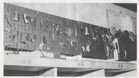
Keeping a parts room stocked with the proper jacks, sinkers, needles, sliders, screws, cams, coil springs and gears is a problem in any knitting room. This problem becomes greater in a plant remote from the machine shop which supplies the parts.
