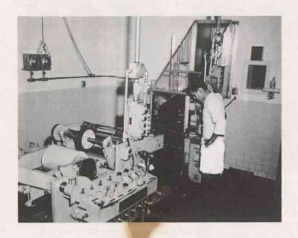
must be adjusted with utmost precision to assure a uniform oxide coating thickness throughout the entire width and length of the roll.
