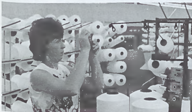
Some textured polyester yarns go into special programs that require precise quality characteristics. After texturing, a sample from each package is knitted, dyed, and tested to insure that proper specifications are met. Lucy Pridden is shown setting the yarn up for knitting.
