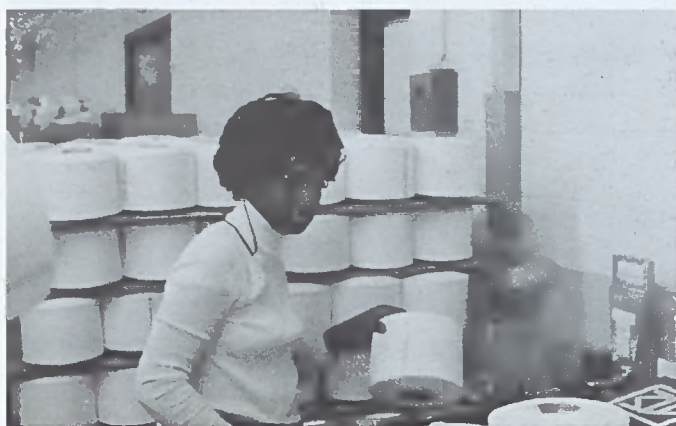
As yarn is sent from the Texturing Plant to the Dye Plant, it is classified into groups according to size and weight of the package. Juanita Wilson inspects the yarn and assigns it to the proper classification.
