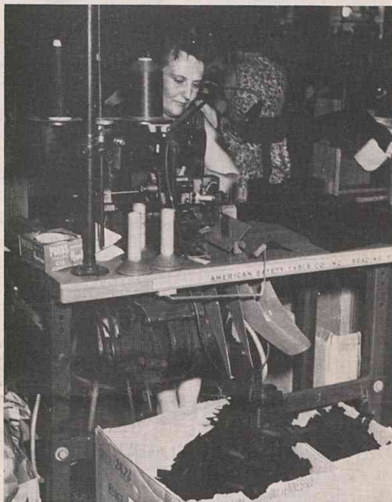
NEW BELT LOOP MACHINE — Agatha McDonald is shown operating the new belt loop machine which the engineering department says is resulting in a great saving of material.
