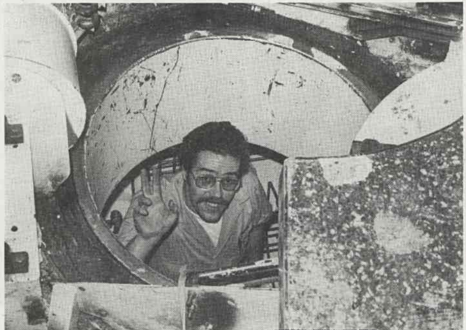
DOWN THE HATCH —John Boyce of Oceaneering International Inc. disappears into the Hyperbaric Chamber's "wet pot" to prepare a work project for the divers who will participate in the high pressure experiment scheduled to begin next week. The ergometer he is setting up will help scientists measure the work efficiency of divers using different types of breathing gear. (photo by Dale Moses)
