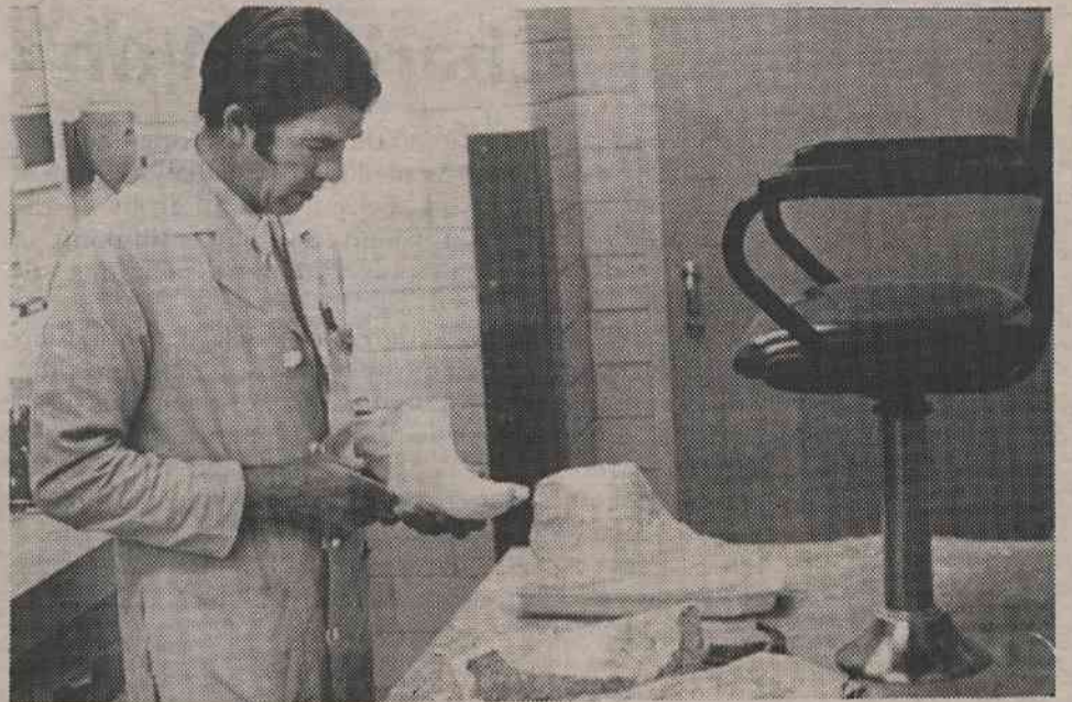
BEGINNINGS OF A SHOE —Felton Elliott has broken the mold from around the cast of a patient's foot. From this cast and the one for the other foot, he will make special shoes to fit the patient's misshapen feet. The Limb and Brace Shop, one of a number in the country, has helped numerous amputees resume almost normal lives.
