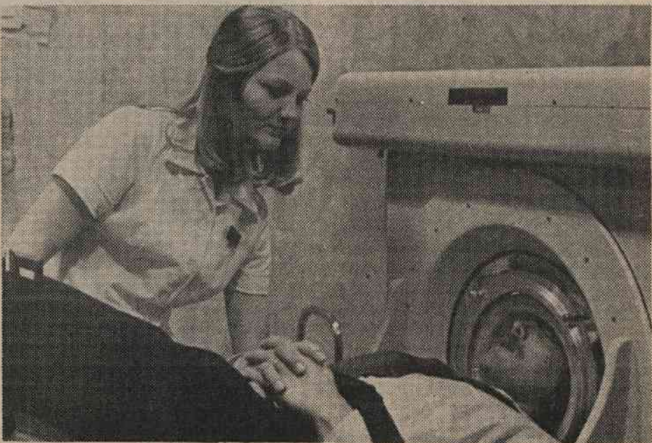
NO, IT'S NOT A WASHING MACHINE —Neuroradiology technical supervisor Brenda Warwick adjusts the Department of Radiology's new CCT scanner, a $440,000 diagnostic device for detecting tumors and other diseases of the brain. The "patient" is Intercom editor Dave Williamson. (Photo by Sally Herndon)
