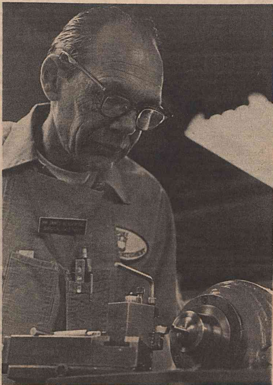
DELICATE WORK —Craftsman James Blackwood alters a nozzle to handle larger surgical suction tubes than those furnished by the manufacturer. The Surgical Instruments Shop can modify commercially available equipment or build new items to meet physicians' specifications. (Photo by Jim Wallace)
