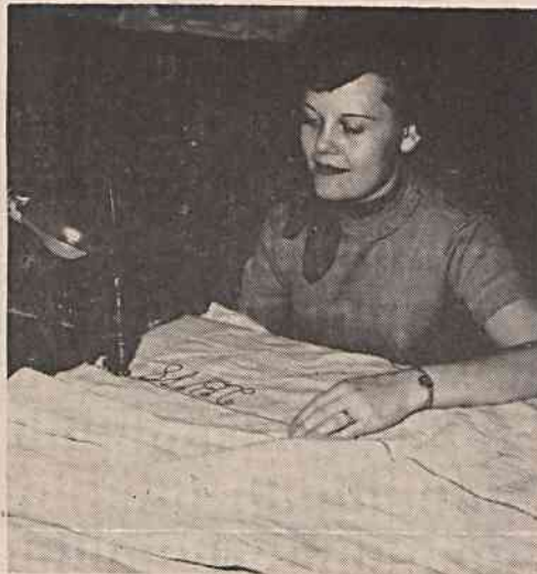
IN CLOTH ROOM , number corresponding with number on loom ticket is sewed on header cloth by machine operator Leona Spencer.
